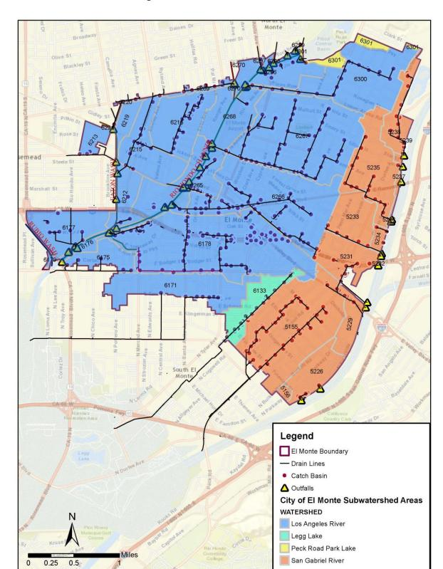
Figure 1-6: Catch Basins and Drain Lines
